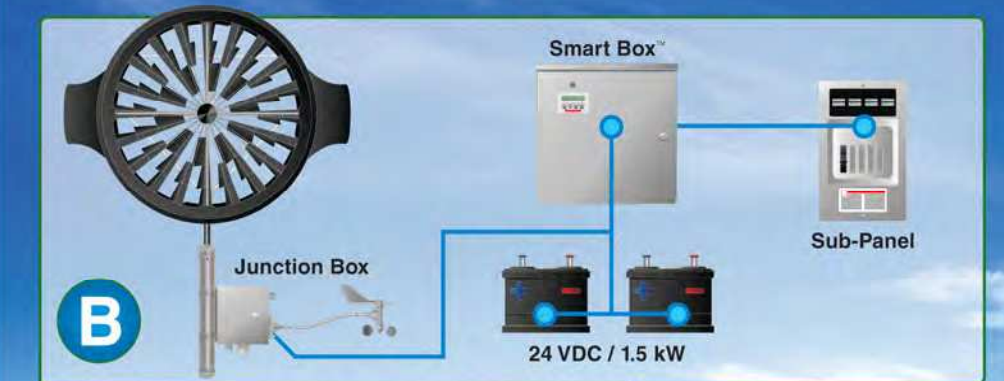
Non-Grid Tie connects to the building subpanel
